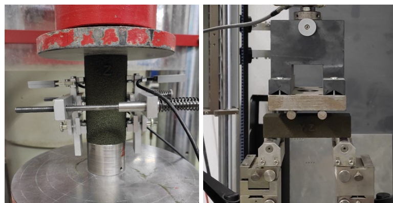
Figure 7. Left, Uniaxial compression tests and axial extensometer. Right, Four point bending test.
