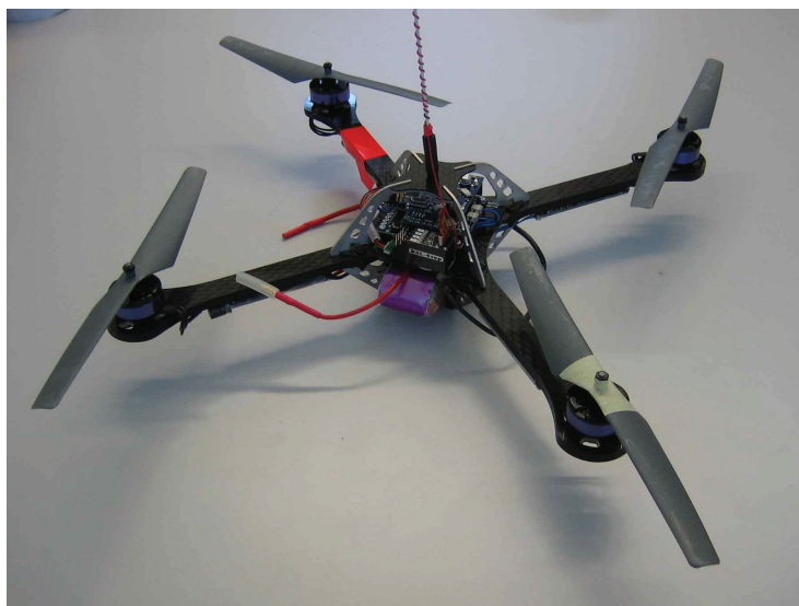
Figure 2. The quadrocopter, measuring 53 cm in diameter.
