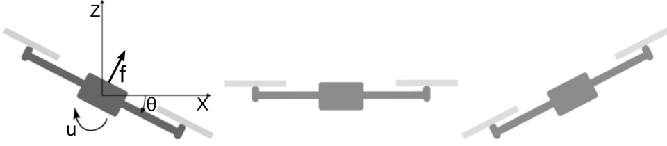
Figure 3. The desired side-to-side motion, a schematic of the two-dimensional quadcopter model.
