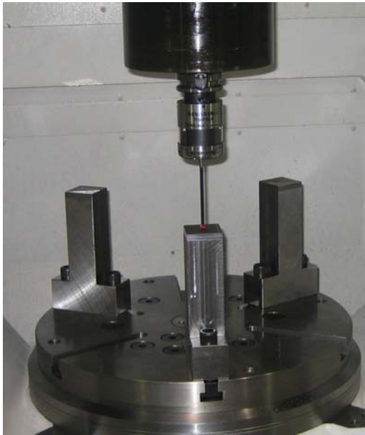
Fig. 13. Setup of three artifacts to calibrate translational and tilt error motions of rotary axes [153].
