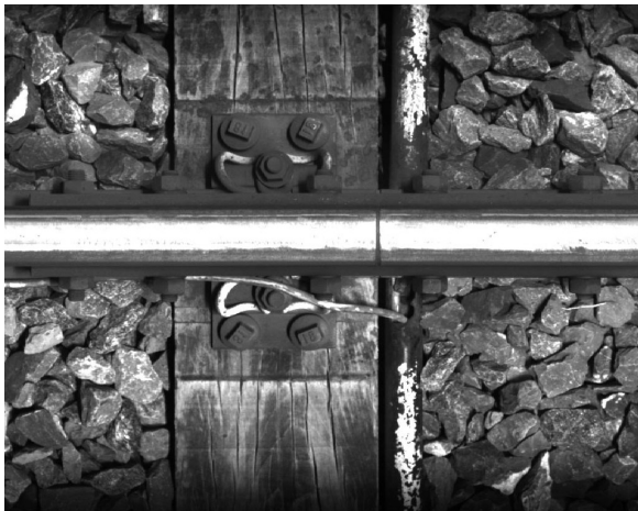
(a) Intact insulated joint
