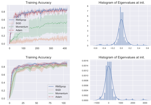
Figure 24: (Top row) Training Fashion-MNIST (Xiao et al., 2017) on a narrow (32 hidden units per layer) 128 layer ReLU MLP with He init. Learning rates are grid-searched (best is shown). Plotted are mean and 95% confidence interval of 10 random seeds. See the appendix in Orvieto et al., 2022b for hyperparameters and test accuracy. Note that RMSProp successfully trains despite the fact that both gradients and curvature vanished. Yet, as can be deduced from how gradient norms evolve over time, SGD struggles to escape the flat plateau which is not surprising given that the negative eigenvalues are very small. (Bottom row) Training Fashion-MNIST on a wide (128 hidden units per layer) 128 layer ReLU MLP (He init.) Training accuracy and gradient magnitude over epochs as well as eigenvalues at initialization. Increased width prevents vanishing and allows SGD to train.
