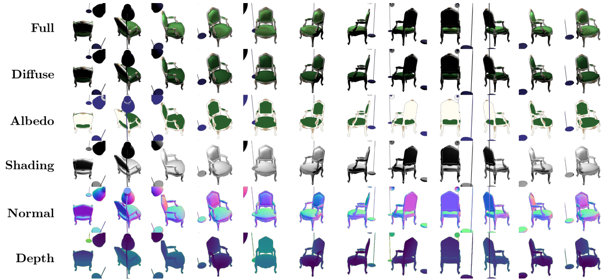
Figure 3.1: Overview of the Intrinsic Dataset showing several samples from the test split of the Chair scene. From top to bottom: Full colour render, Diffuse render conforming to the Lambertian assumption, Albedo, Shading (excluding shadows and self-shadowing), Camera-space normal, and Depth map passes. Samples which focus on auxiliary objects, not shown for clarity.
