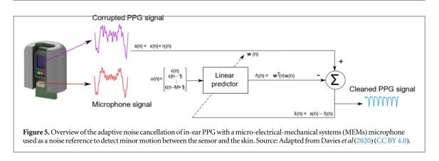
canal derived physiological signals. To this end, micro-electrical-mechanical systems (MEMs) microphones, capable of detecting minor movements between the sensor and skin, have proven effective at removing these ear-specific motion artefacts from ear-EEG (Goverdovsky *et al* 2015). By the same principle, the use of MEMs microphones may provide an effective artefact reference and thus enable a stable 24/7 in-ear PPG trace. This principle is outlined in figure 5.
