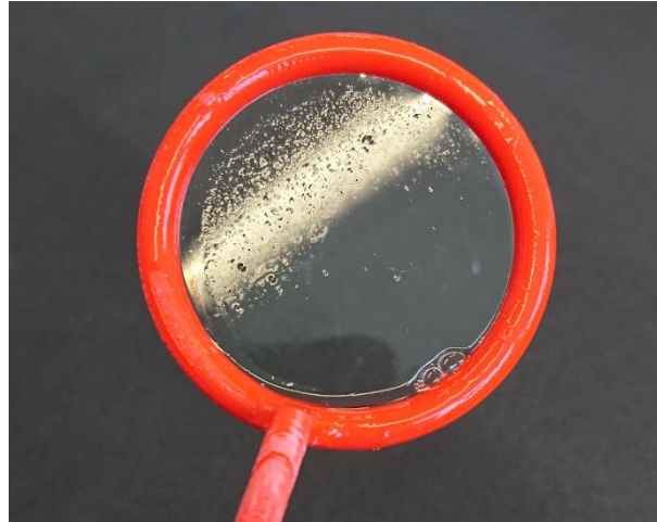
Figure S1: Photography of the loop with a HEWL amyloid 2D foam film at pH 8, showing inhomogeneity due to aggregation.
