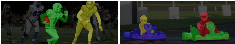
Figure 2.2 – Two examples of Video Object Segmentation visually represented with the help of a different semi-transparent colored overlay per target ( foreground ). Everything else in the scene is considered as background .
