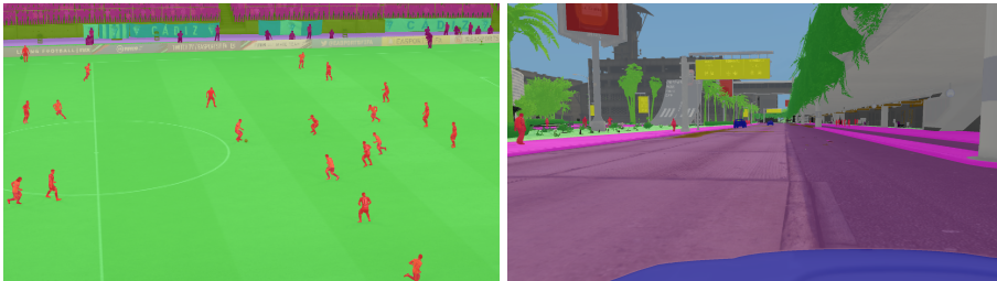
Figure 2.1 – Semantic Segmentation visually represented with colored overlays on the original images. Each semi-transparent colored overlay represents a different class. Each situation has a different set of pre-determined classes: on the left a football game and on the right a typical autonomous driving situation.
