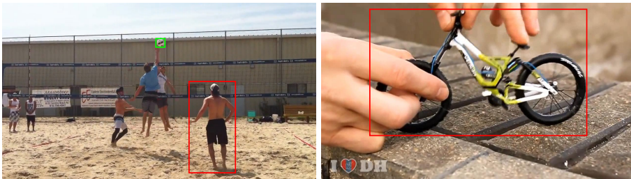
Figure 2.4 – In Visual Object Tracking, a target is defined by a bounding box. Simple targets like the volleyball (□) are very well defined by this representation. In contrast, more complex objects like the volleyball player or the bike (□) can only be represented well in terms of location in the image. A big part of the content inside each bounding box does not belong to the target object.
