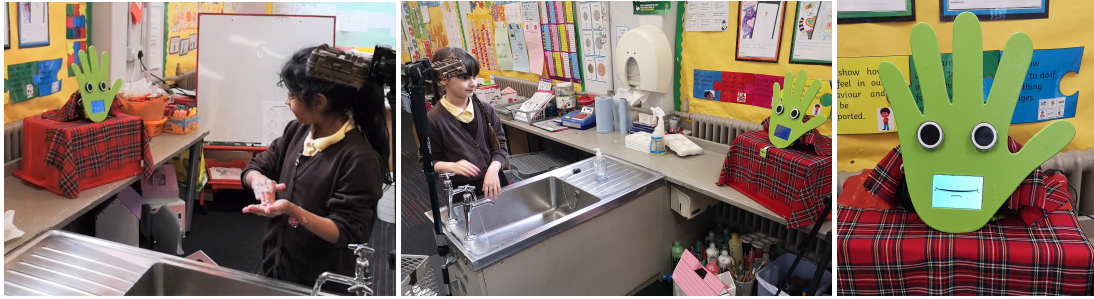
Fig. 1. WallBo giving 1:1 instructions to the pupil near handwashing station about 10 steps of handwashing (left), WallBo (right)
