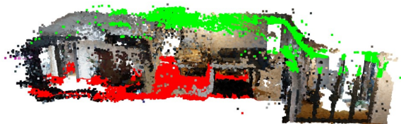
Figure 42. Top (green) and bottom (red) plane in the point cloud
