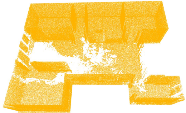
Figure 53. CAD model point cloud, points near captured data removed
