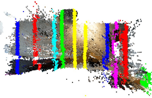
Figure 77. 10 planes found by the constrained RANSAC approach
