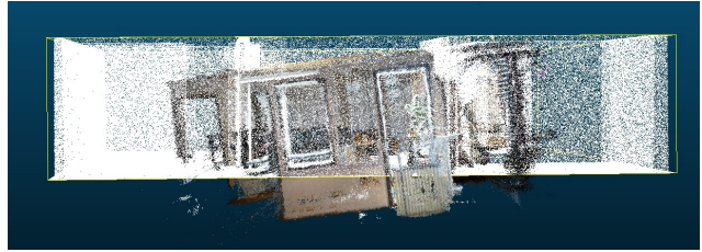
Figure 82. Result for ICP with scaling disabled, side view
