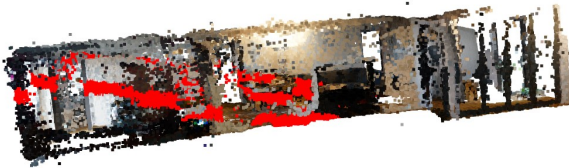
Figure 9. Unusable plane found by the RANSAC algorithm
