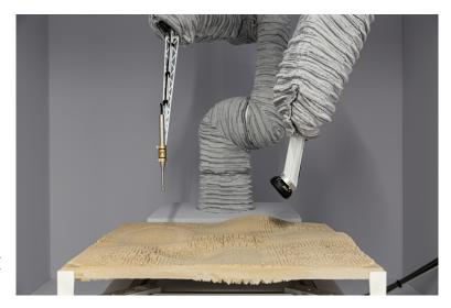
**Figure 2.4:** A closeup view of the data acquisition setup. The microphone (left) and speaker (right) endeffectors attached to two Stäubli TX2-60L robots.
