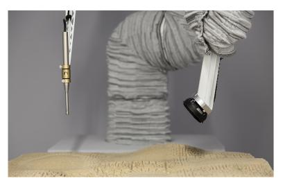
Figure 3.4: Microphone (left) and speaker end-effector (right). The microphone is attached to an acoustically transparent steel mount, and the speaker is tilted to optimise directivity and ensure robot reachability.
