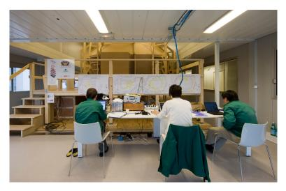
Figure 1.6: Exterior view of the 1:10 physical scale model of the La Philharmonie de Paris during an acoustic measurement. ©Nicolas Borel.
