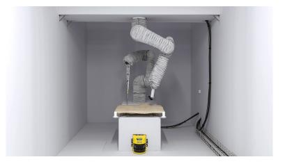
**Figure F.1:** Acoustic data acquisition setup from the DDAD project with two Stäubli TX2-60L robots in an acoustically shielded and absorbent room. The double-sided 3D printed panel of dimensions 585x585 mm is placed in a special fixture [40]
