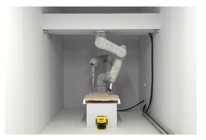
**Figure 3.1:** Acoustic data acquisition setup with two Staubli TX2-60L robots in an acoustically shielded and absorbent room.
