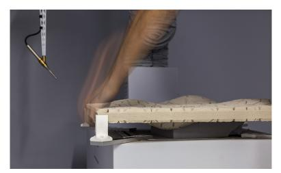
**Figure 3.2:** Double-sided 3D printed panel placed in a special fixture.
