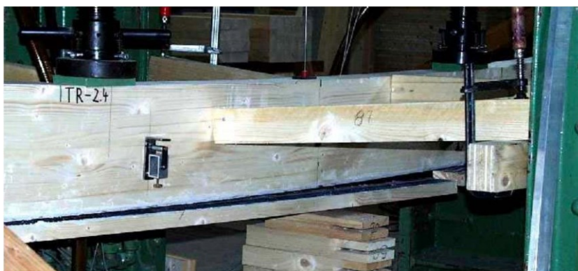
Fig. 11 Reinforced glulam beam, under loading test at University of Karlsruhe (TH). Thin carbon FRP and aramid FRP were used as reinforcements. 104
