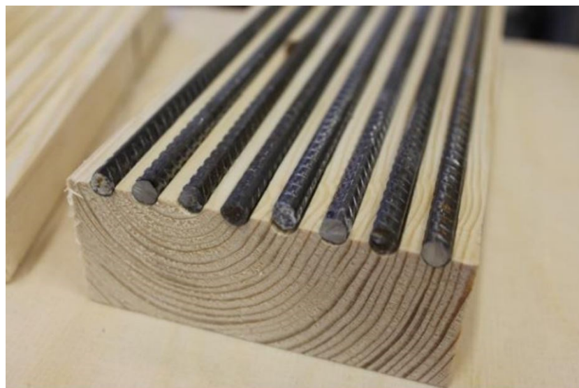
Fig. 14 Glued laminated timber beams reinforced with strands. A research project between different universities in Latvia, 2017. 106
