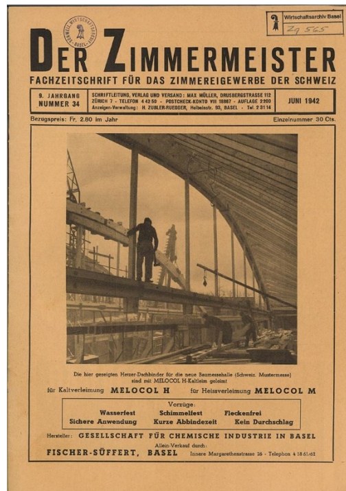
Fig.4 Advertisement for the synthetic glues developed by CIBA, appearing on the cover page of the Association of Swiss Mastercarpenters' journal. This glue was used for the glulam structure of the building of the Trade Fair of Basel in 1943.
