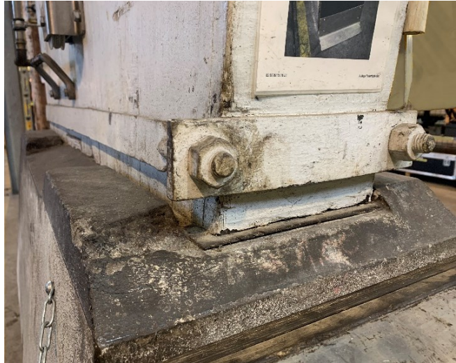
Fig. 18 Detail of a steel column connection to a concrete foundation by means of a slightly curved metal sheet to reproduce the hinge effect. (Königer, Otto, Die Konstruktionen in Eisen , 1902)
