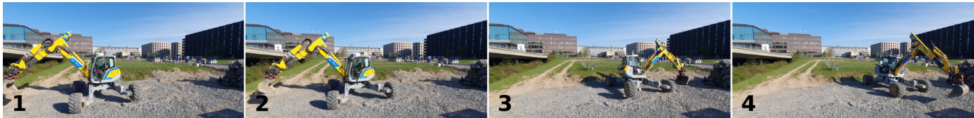
Fig. 23: HEAP performing a stepping turn and moving laterally. The chassis keeps the azimuth approximately the same as at the beginning of the maneuver.
