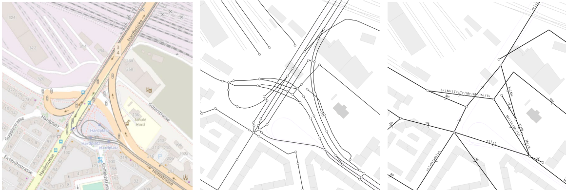
1 2 Figure 3: OSM map preview (left), raw street graph (middle), and simplified street 3 centerline graph (right) at Zurich-Hardbrücke
