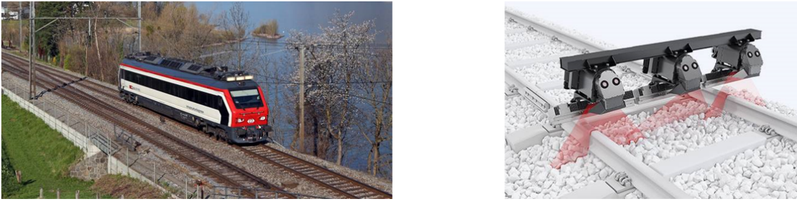
Figure 7.1: Diagnostic vehicle and illustration of monitoring system
