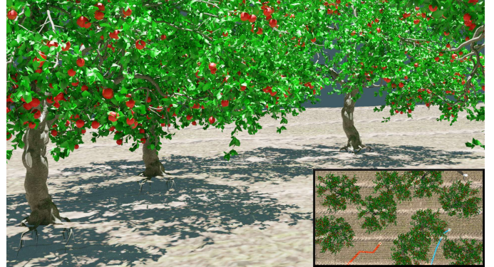
Fig. 1: The view of one of two drones exploring a synthetic forest with geometrically realistic tree models. The inset depicts the top view of the scene of the experiment and parts of the robots' trajectories. The proposed system guides the safe and successful exploration of the digital model of the forest by the two UAVs. The planner is able to avoid collisions between the UAVs and the scene while clearing frontiers on the go by balancing cautious and aggressive navigation in a bid to maximize the efficiency of the exploration. Coordination is achieved in a decentralized fashion, relying on direct peer-to-peer communication.
