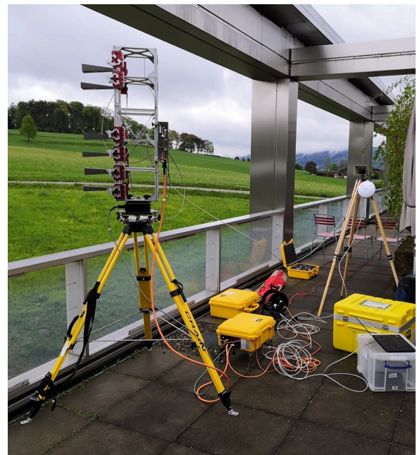
FIGURE 2.3: Bistatic KAPRI device configuration (left: primary device (P) equipped with narrow-beam slotted-waveguide antennas and right: secondary receiver device (S) equipped with horn antennas). Reference link horn antennas are placed on tripods on the right side of the two images, together with long-range Wi-Fi antennas for remote device control.
