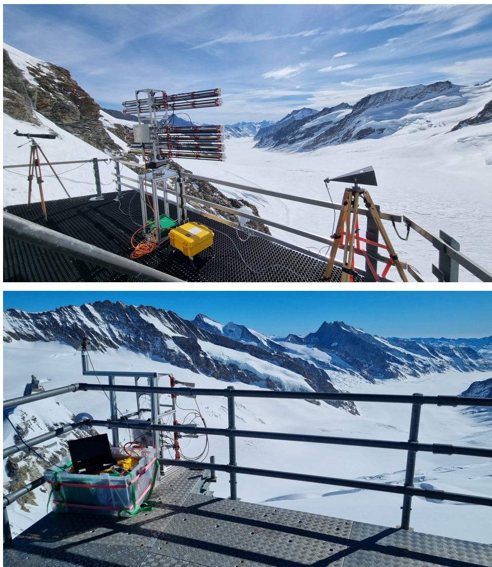
FIGURE 3.1: Photos of both devices deployed at the High Altitude Research Station Jungfrauoch complex. The primary device (top) was deployed on top of the Research Station terrace, the secondary device (bottom) was deployed on the terrace of the East Ridge ( Ostgrat ) building. Both devices observe the Jungfrau area, visible in the background of both images. The synchronization antennas pointed along the bistatic baseline are visible in bottom right and top left parts of the two images respectively.
