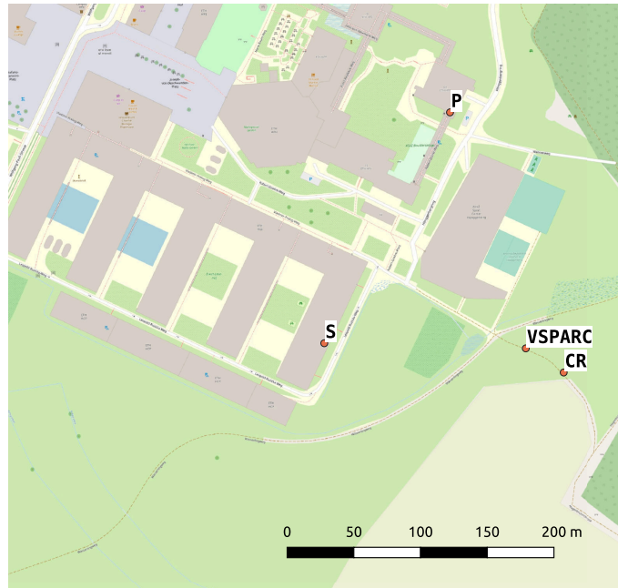
FIGURE 2.11: Synchronization link experimental setup. The bistatic reference signal is transmitted between the primary (P) and secondary (S) devices along a \sim 200 m bistatic baseline. Map data © openstreetmap.org contributors.
