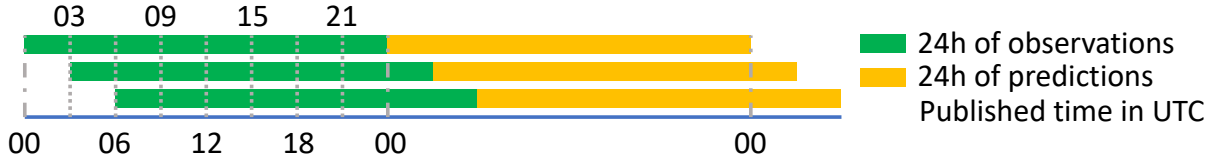
Figure 2.1: Schematic diagram of the IGS Ultra-rapid orbit products provided by GFZ
