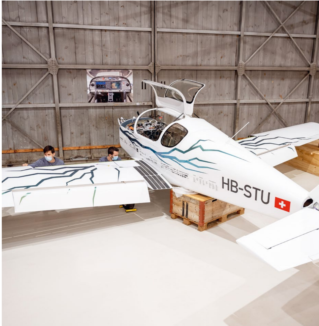
The "e-Sling" focus project involved eight ETH students working on an electric aircraft powered by batteries and hydrogen. For a whole year, Hangar 3 at the Innovation Park in Dübendorf, Zurich, was the centre of their lives. (photo: ETH Zurich / Daniel Winkler)
