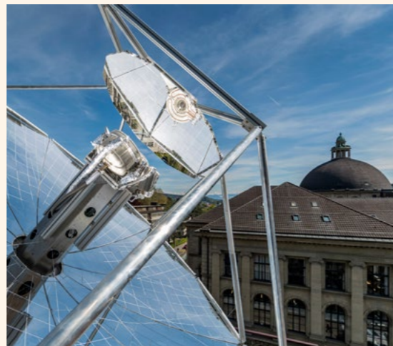
Experiments in renewable energy systems, such as this solar mini-refinery, are under way on the roof of ETH Zurich's Machine Laboratory. (photo: ETH Zurich / Alessandro Della Bella)
