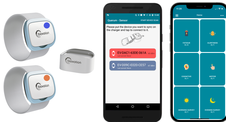
Figure 7.1.: Study methods for in-the-wild study phase: two color-coded everion devices for continuous monitoring of physiological data with one charger(left), stationary phone for everion data download and sync (center) and crónico app for gathering ground truth feeling.
