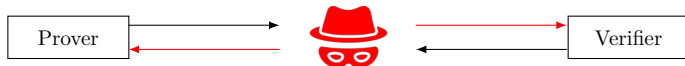
Figure 2.1: Mafia Fraud attack scenario against secure ranging. The attacker is located between prover and verifier and does not possess any knowledge of the cryptographic material.
