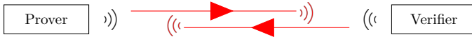
Figure 2.5: Relay attack: The attacker establishes a communication path between prover and verifier. Using amplification and a wired or wireless connection, the attacker can bridge an arbitrary distance and circumvent any propagation obstacles of the actual channel.
