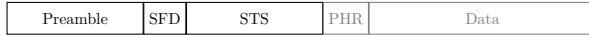
Figure 4.4: HRP Frame Structure: The cryptographically generated Scrambled Timestamp Sequence (STS) occurs after a publicly known preamble and Start-of-Frame Delimiter (SFD).
