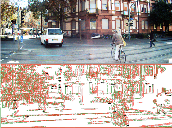
Figure 7.2: Top: An unrectified image from the KITTI dataset [19]. Bottom: For illustration purposes, canny edges detected from correctly (in green) and incorrectly (in red) rectified images are shown. A set of incorrect rectification parameters results in pixel projections from the raw image to be displaced relative to that with the correct parameters (indicated by the black segments). The mean of the L2-norms of these displacements over the image corresponds to the APPD.
