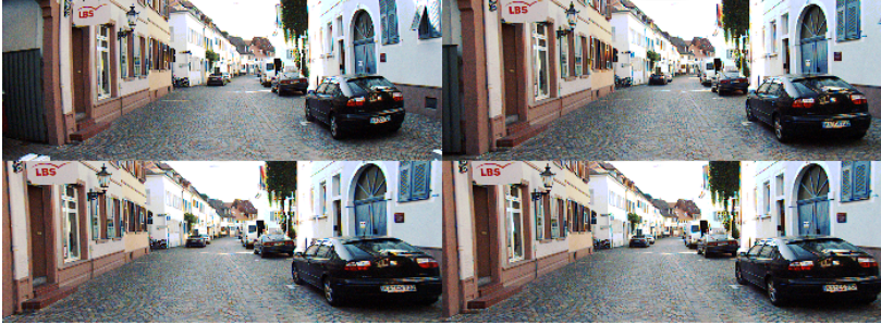
Figure 7.1: Illustration of the subtle differences that a miscalibration detection system needs to be sensitive to. Top left: Unrectified image; Top right: Correctly rectified image; Bottom: Two examples of incorrectly rectified images. The image is taken from the KITTI dataset [19].
