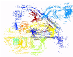
(c) Globally consistent and optimized multi-session map in a disaster rescue training area.
