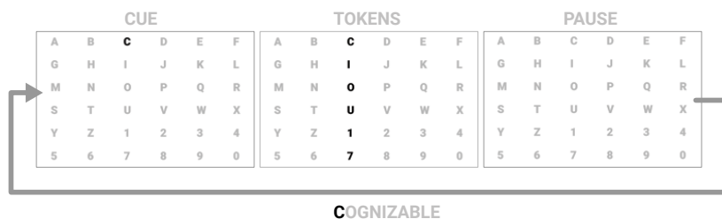
FIGURE 34: General sequence of the spelling session for a given word (here: COGNIZABLE). For each character, the three main steps occur successively. 1). Left: Cue, The character to spell is shown for a fix amount of time. 2). Middle: Tokens, a random sequence of rows and columns is flashed with fixed periods of flashes and non- flashes. 3). Right: Pause, a short non-flashing period of time occurs before going to the next character to spell while applying the same sequence until the last character.
