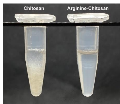
Figure S9.1 | Solubility of chitosan and arginine-chitosan. Unmodified chitosan (left) is not soluble in PBS at neutral pH and forms clear precipitates. In contrast, Arg-Chi (right) is nicely soluble at neutral pH, resulting in a clear solution with no precipitation.
