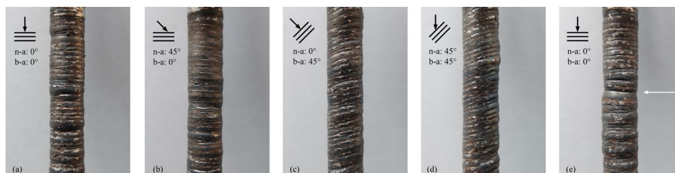
Figure 3.47: Surface quality of printed bars with different building and nozzle angles from Michel et al., 2022.
