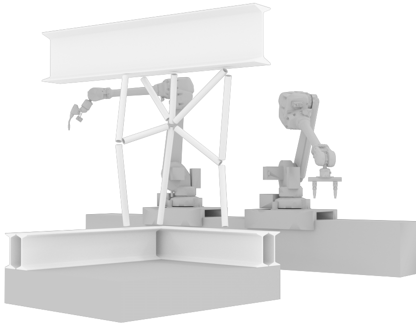
Figure 5.40: Robotic assembly setup with welding robot on the left and assembly robot on the right (in gray) and unconnected elements of the base structure (in white).
