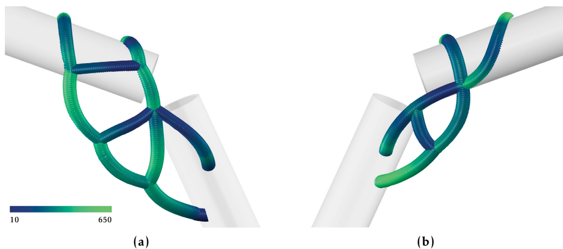
Figure 5.24: Reachability of paths calculated for the ladder graph search: greener sections of the paths are more reachable than blue sections. The lower bound is set to 10 reachable orientations; the upper bound is 650 reachable orientations, from an original pool of 1199 frames to test per point. On greener sections, more tool orientations are possible than on blue sections. Blue sections, the less reachable sections of the paths, influence the overall results of the ladder graph search.
