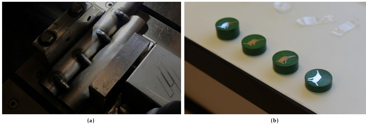
Figure 3.40: Primitive connections process: (a) Specimens before cutting, and (b) Specimens after hot-mounting.
