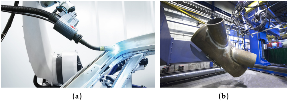
Figure 2.8: Welding: (a) Different welding methods used in car assembly: spot welding and a curved seam performed with the GMAW-based Cold Metal Transfer (CMT) process by Fronius, Photo: Fronius, Audi Robotics, and (b) Welding of a K-node of an offshore oil jacket structure. Photo: PEMA Welding.
