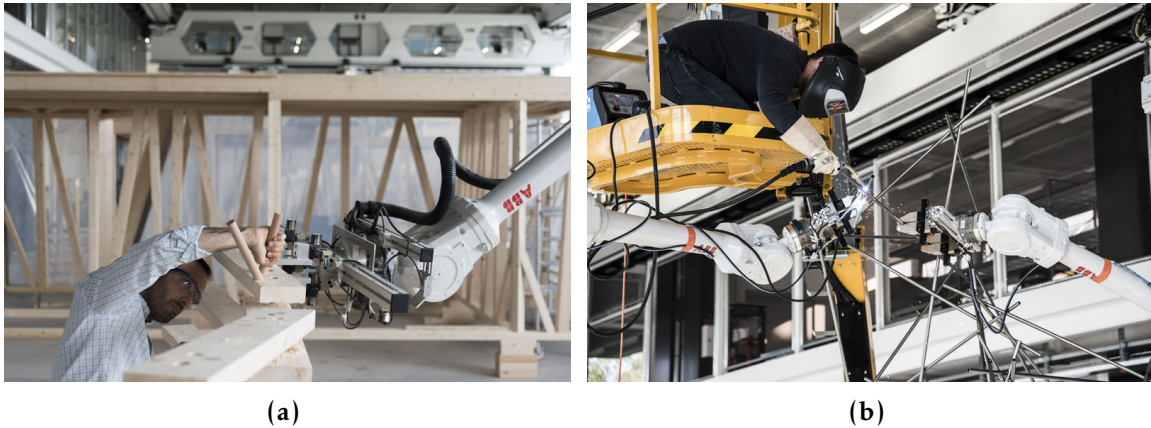
Figure 1.4: Manual joining for robotic assembly: (a) Gradual Assemblies: insertion of wooden dowels (2018), Photo: Andreas Thoma, and (b) Lightweight Metal Structures: welding (2018), Photo: Martin Rusenov.
