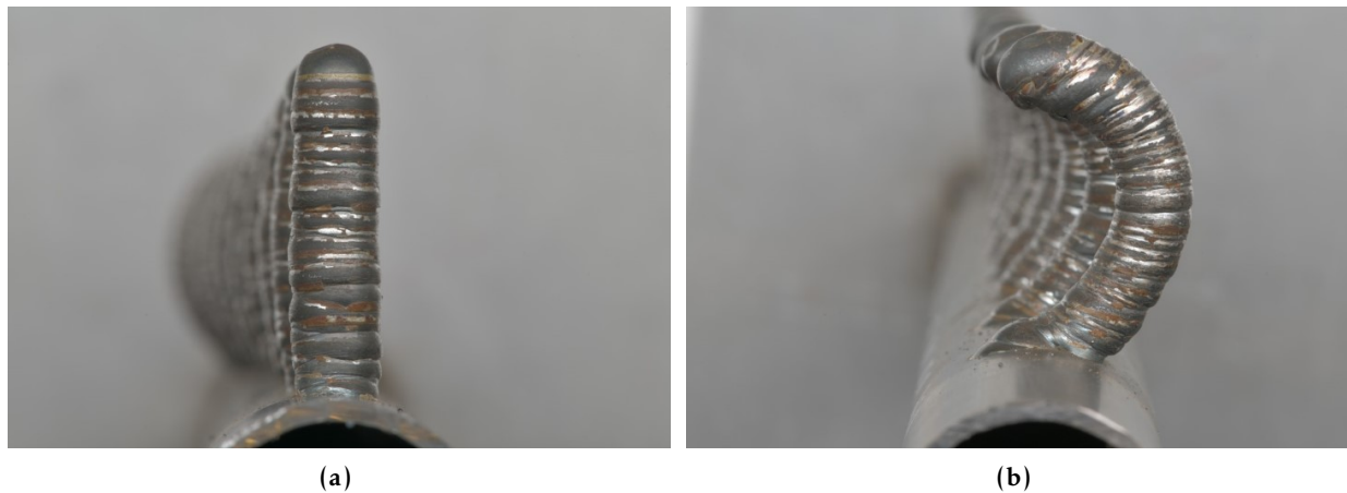
Figure 3.35: Curvature results: (a) Zero curvature, and (b) Maximum curvature
