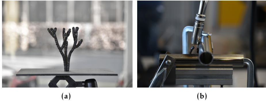
Figure 3.9: WAAM vs. IPWAAM: (a) freestanding, and (b) collision constrained.
