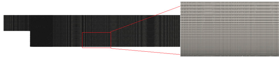
Figure 3. General view of the grid and zoom of the grid near the bottom wall.
