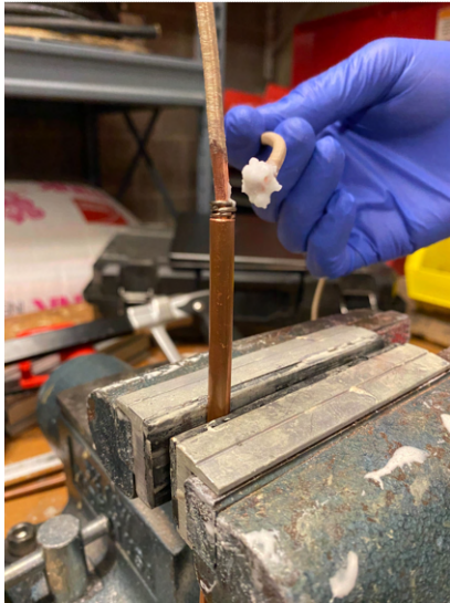
Figure 56: Picture a) depicts the preparation for brazing the end of the square wire to a swage-lock-able copper tube. The fiberglass insulation is stripped, and the copper is fitted to the tube. Then flux and solder are applied to the joint before heating it with a propane torch. Image b) depicts the initial plan of mounting water-cooled coils inside the reentrant viewport, close to the atoms. It was abandoned due to the lack of access to the objective and inhomogeneity concerns.
