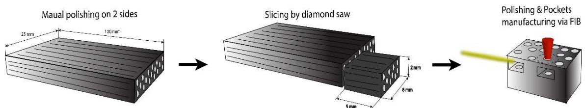
Figure 1: Micromechanical specimen preparation and workflow (not to scale). Left : The top ( 25 \times 100 \text{ mm}^2 ) and side ( 25 \times 2 \text{ mm}^2 ) faces are manually polished. Middle : micromechanical sample is sliced. Right : The sample is mounted on an SEM stub (not shown) and a pocket is milled via FIB.
