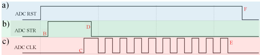
Figure 6.5: ADC control signals: a) ADC reset operating on inverse logic, b) ADC start conversion operating on inverse logic, and c) ADC clock highlighting the track phase and the successive conversion steps. Figure adapted from [11].
