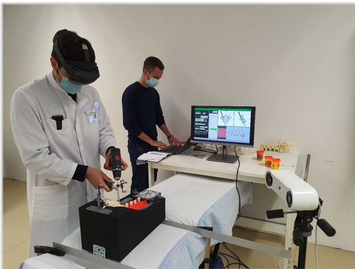
Fig. 22: Experimental setup showing the participant navigating with HoloLens 2, the spine bed, tracking camera and external screen.
