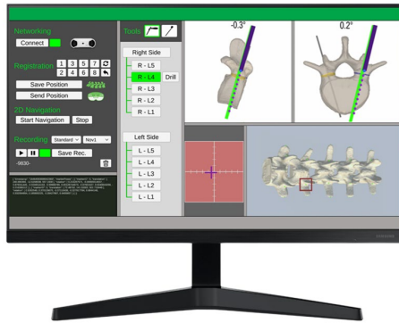
Fig. 20: Standard navigation with user interface to connect to the external tracking camera, start recordings and select a vertebrae (left), a top view on the segmented spine model (bottom right), a magnifying view for fine-positioning of the tool tip on the entry point (red area in the middle), and 2D slices in sagittal and transversal direction (top right).
