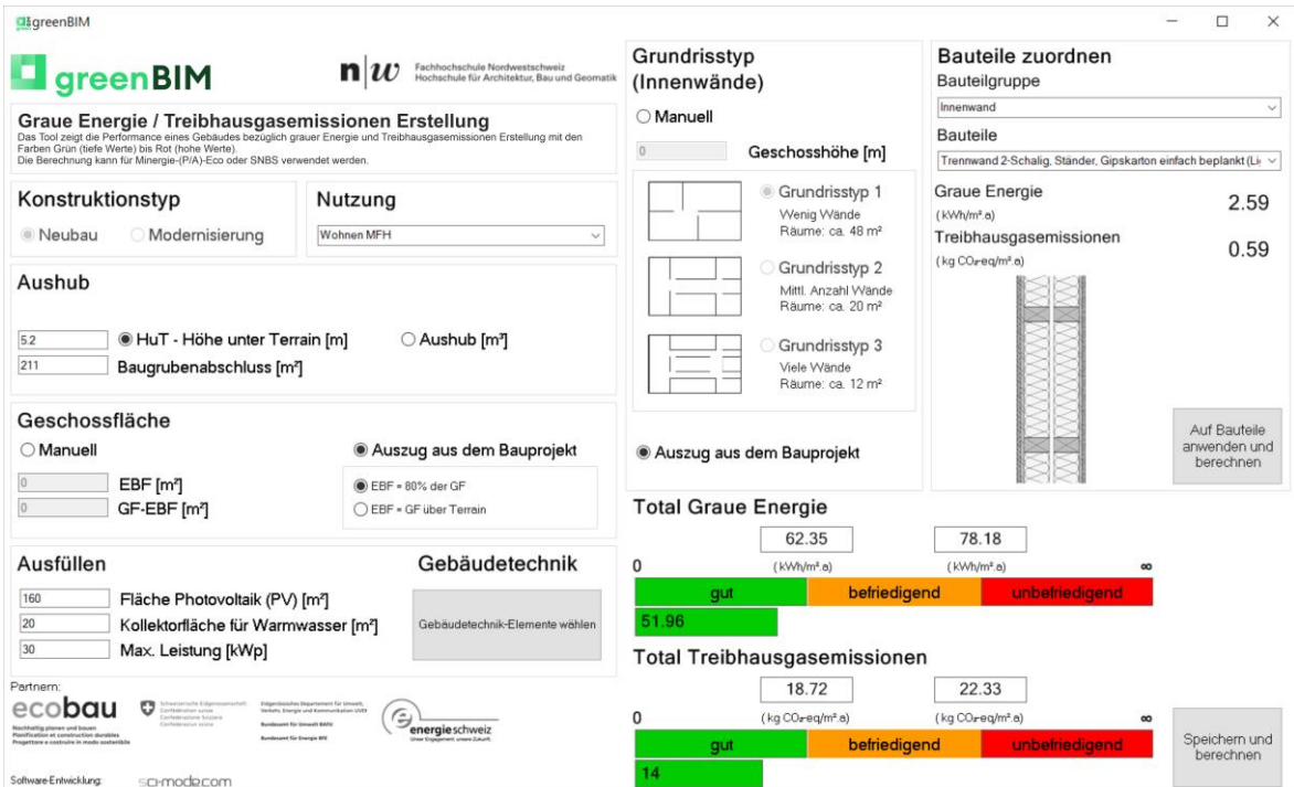
Figure 14: Cockpit of the greenBIM tool (Revit version) with guidance through the inputs and direct result output. Source: [14]
