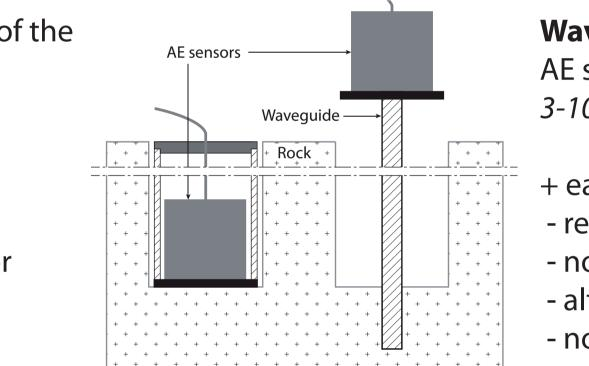
Waveguide: thin rod transmits AE signal to sensor at surface 3-10 dB loss + easier to install - reduced data quality - not protected - alteration of field site - no constant coupling
