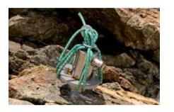
April 2010, Jungfraujoch, Switzerland (Amitrano et al. 2012) • Outdoor measurements with lab equipment during 4 days • Piezoelectric sensors and six-channel high-frequency board Proved the potential and feasibility of AE measurements in PermaSense
