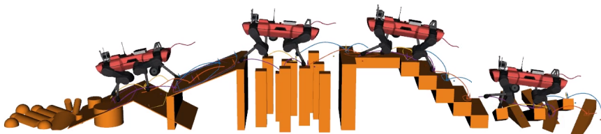
Figure 6.10: ANYmal traversing an obstacle course in simulation. Snapshots are shown for a the traversal with a trotting gait at 0.8m/s. The MPC predictions are shown for each foot and for the torso center. For all contact phases within the horizon, the convex foot placements constraints are visualized.
