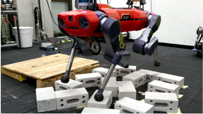
Figure 5.1: ANYmal (Hutter et al., 2016) performing a trotting gait on stepping-stones.
