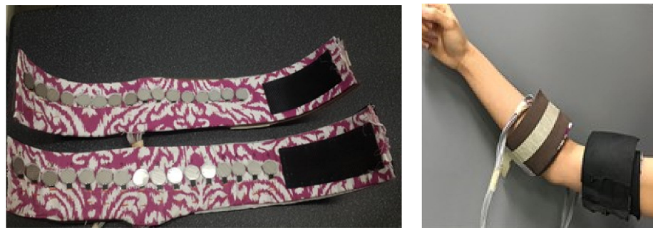
Figure 1. Two customized force myography (FMG) bands worn on the forearm and upper arm muscle belly of a participant to read muscle contraction.
