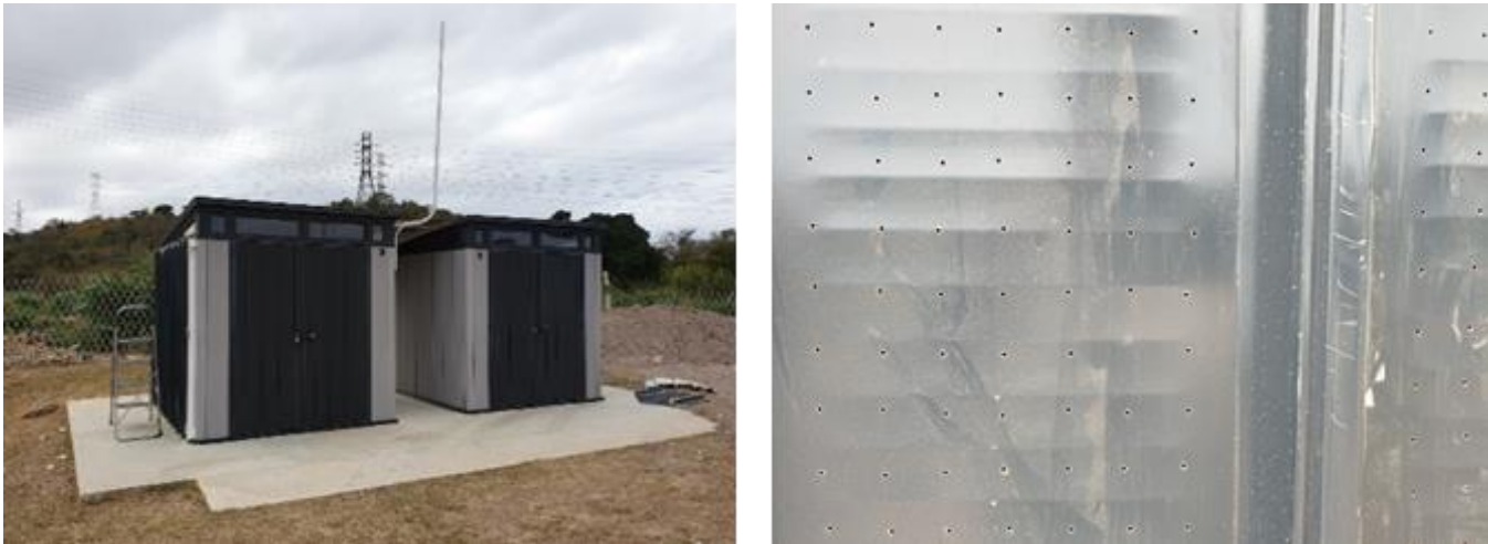
Figure 3.17. A pilot-scale solar dryer developed by Swansea University and tested in Durban, South Africa. Above: sludge is placed inside these sheds to dry. Below: the walls of the sheds absorb solar energy and transfer it to the sludge inside through a ventilation system (photos: UKZN PRG).
