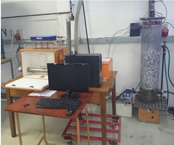
Figure 3.19. Left: the custom-designed convective drying rig (photo: UKZN PRG) and right: a schematic representation of the convective drying rig, F: air-flow measurement; T: temperature measurement; M: mass measurement; HR: relative humidity measurement.
