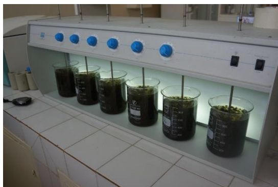
Figure 3.5. Example of a jar test setup to test suitability of a conditioner (photo: Sandec).
