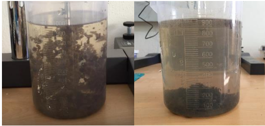
Figure 3.4. Above: steps in faecal sludge conditioning, coagulation, flocculation, and sedimentation; below left: flocculation of faecal sludge; below right: settling of faecal sludge flocs (figure adapted from Ward and Strande, 2019, photos: IHE Delft).
