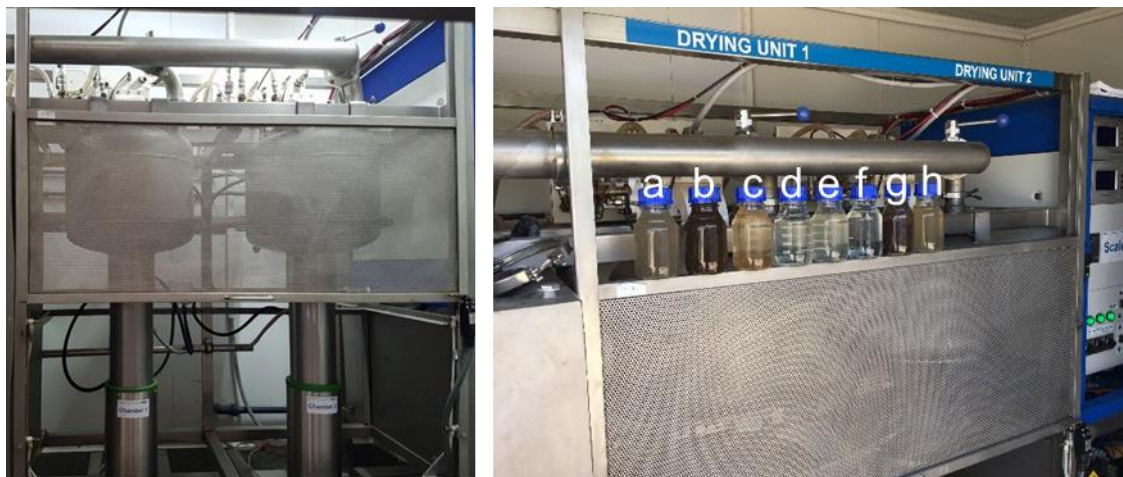
Figure 3.24. Left: an experimental microwave-based faecal sludge drying unit, and right: samples taken at different points in the process: a) filtrate from the sludge press, b) concentrated sludge from the sludge press, c) ultrafiltration concentrate, d) ultrafiltration permeate, e) reverse osmosis concentrate, f) reverse osmosis permeate, g) dry sludge, and h) condensate (photo: IHE Delft).
