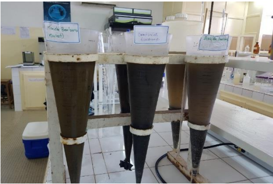
Figure 3.6. Example of an SVI settling test setup with graduated Imhoff cones (photo: Sandec).
