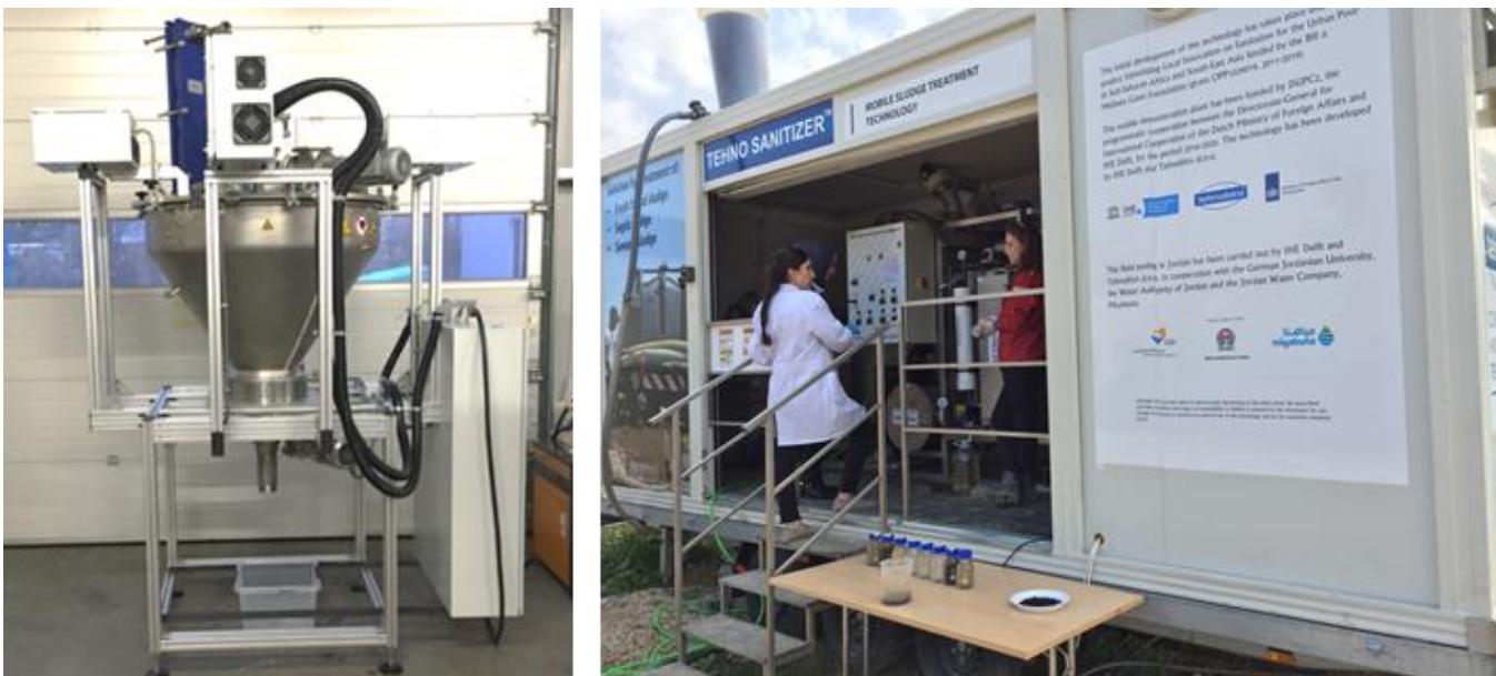
Figure 3.18. Left: the bench-scale Shit Killer microwave-based technology for sludge treatment developed by IHE Delft and Fricke und Mallah Microwave Technology GmbH, and right: the follow-up prototype – the pilot-scale Tehno Sanitizer developed by IHE Delft and Tehnobirot d.o.o. (photos: IHE Delft).
