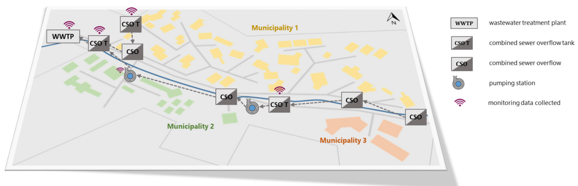
Figure 1.1: Simplified example of an urban water system with a WWTP and several CSO tanks, CSOs, and pumping stations. In the example, monitoring data is collected for selected urban water system elements.
