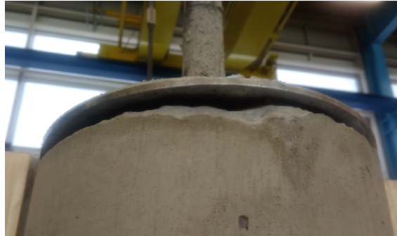
Figure 5.6. Voids created while casting at the top end of column D.
