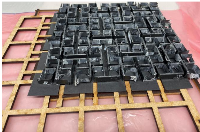
Bonding stacks and metastructure
