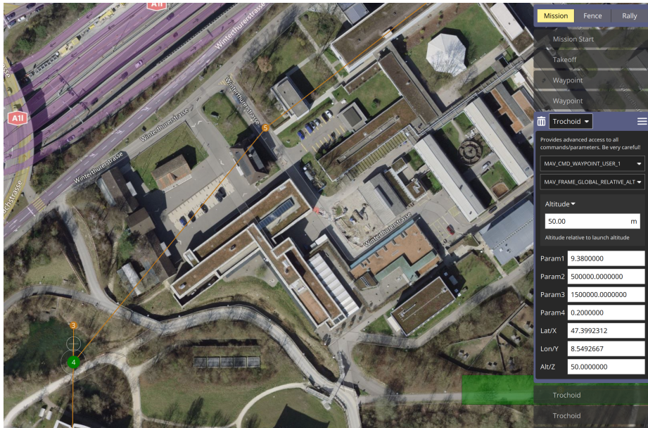
Figure 6.3: Example mission with a three segment trochoid path (CCC) represented by three separate trochoid waypoints in QGroundControl.
