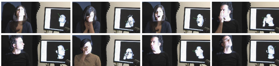
Fig. 14 Example frames from our real time head pose estimation system, showing how the regression works even in the presence of partial occlusions, notably of the nose. Facial expressions also can be handled to a certain degree, even though we trained only on neutral faces
