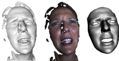
Fig. 24 Example frame from the B3D(AC)^2 database. High quality range scans come together with RGB texture (not used in this paper) and a high definition generic template deformed to match the facial expression in each frame
