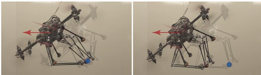
**Figure 7.56:** Experiments with the base following an arc trajectory up to  $45^\circ$ , and the end effector tracking a fixed point, while a disturbance is applied for an active (left) and fixed (right) manipulator. Red arrows represent where the virtual disturbance force is applied, while blue circles indicate the desired end effector position.
