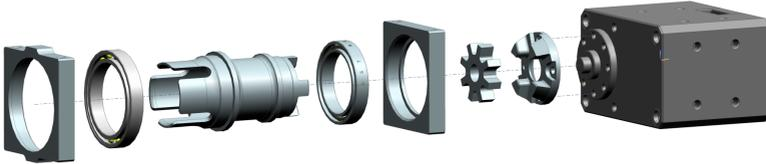
(a) Exploded component diagram of **direct** tilt-rotor transmission.
