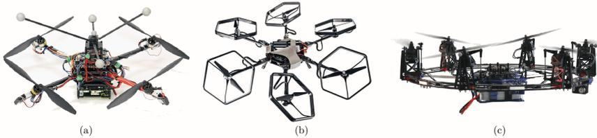
**Figure 1.4:** State-of-the-art in fully actuated tilt-rotor aerial robots. (a) The ‘holocopter’, with four tilt-able rotor groups [99], (b) ‘Voliro’, an omnidirectional system with six tilt-able rotor groups from ETH Zurich [55], and (c) ‘Fast-Hex’, a system with tilt-able rotors coordinated by a single motor from the University of Twente [103].
