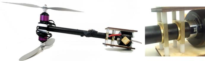
**Figure 6.9:** Physical prototype of the complete double tilt-rotor assembly (left) and a close-up of the power transmitting bearings, isolated from the surrounding structure by nylon stand-offs.
