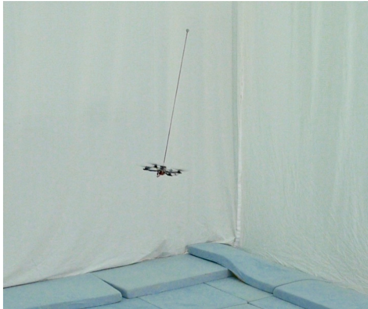
Figure 1. The flying inverted pendulum system used for the experiments presented in this article.
