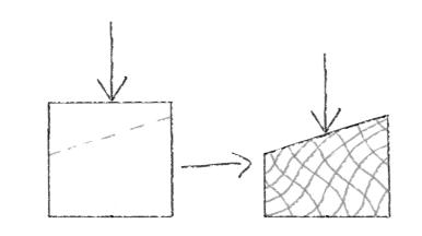
Many AM processes are capable of producing complex structures of small, interconnected geometries, which can be utilized to absorb energy either through elastic or plastic deformation, movement, or controlled breakage.
