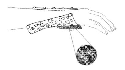
Variable impedance prosthetic socket uses multiple materials to selectively provide support and comfort.
