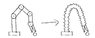
Optimized structural topologies and geometries take full advantage of the geometric freedom allowed by AM. By using the optimized design, artifact mass can be reduced and/or performance can be increased.
