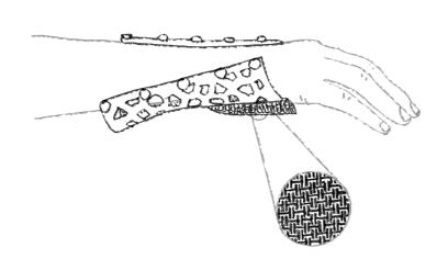
Variable impedance prosthetic socket uses multiple materials to selectively provide support and comfort.
