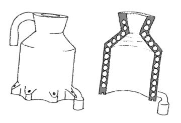
Aircraft duct part reduction from 16 to 1 parts, which now requires no assembly.
