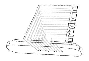
Extrusion die manufactured with AM allows for smoother transions between sections than a milled and assembled die.
