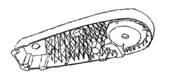
Accelerometer and other circuitry embedded into helmet insert that measures the acceleration of the head.
