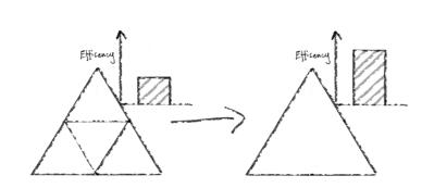
Part consolidation is possible with AM because of the geometric freedom it affords. When parts are consolidated, the design can be more resistant to fatigue and vibrational effects over time due to the elimination of fasteners and stress concentration zones.
