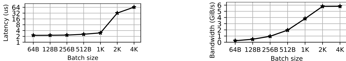
Figure 4.8: Latency and bandwidth of batching 64-byte RDMA Writes. Note log scale of Y axis for the latency plot.
