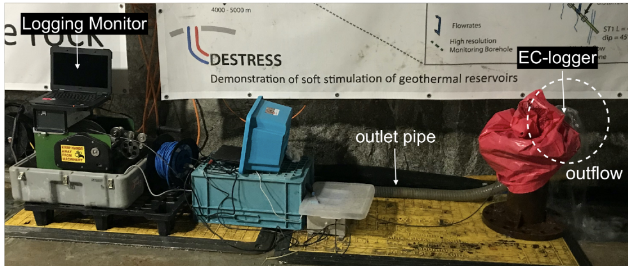
Figure 10: Temporary monitoring set-up during the hydraulic stimulation event on the 23.05.2021, measuring the electric conductivity of the ST1 interval 1 outflow while ST2 was stimulated.
