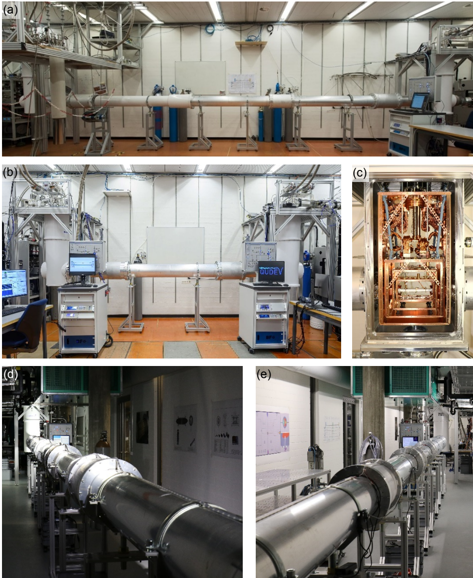
Figure 4.5 Photographs of cryogenic link systems. (a) 10 m link. (b) 5 m link. (c) Intermediate pulse tube cooler used to cool the center of the 30 m link, with side panels of every temperature stages removed. (d) and (e), views towards the opposite ends of the 30 m link.
