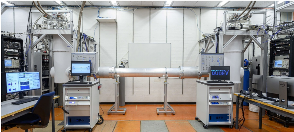
Figure 6.2 Photograph of the experimental setup during operation. The dilution refrigerator units, whose vacuum cans appear as white vertical cylinders, are connected to each other by the cryogenic link (long horizontal aluminum cylinder). The superconducting qubits and the cold waveguide are housed inside the dilution refrigerator units and the cryogenic link, respectively. The electronic instruments are stored in two black racks seen on the far sides of the picture.
