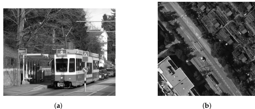
Figure 12. Curbside stops in Zurich. Limiting overtaking, especially when upstream of signalized intersections, can help buses to gain a more advantageous position in the queue when leaving the bus stop. Source: Google maps. (a) Curbside stops for trams and (b) curbside stops for buses with a pedestrian crossing and island next to them.
