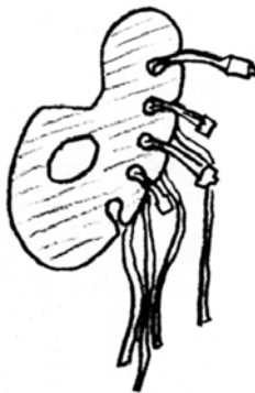
Figure 3: The solution #2 is a “cable palette” in analogy to an artist's palette of paints. Prototyping and testing in the work procedure didn't satisfied the users need of storing and/or shortening the cables.
